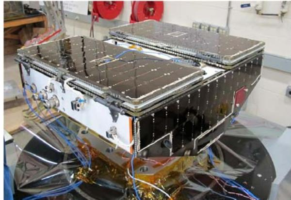
**Figure 12 - CYGNSS Observatory during vibration testing**
