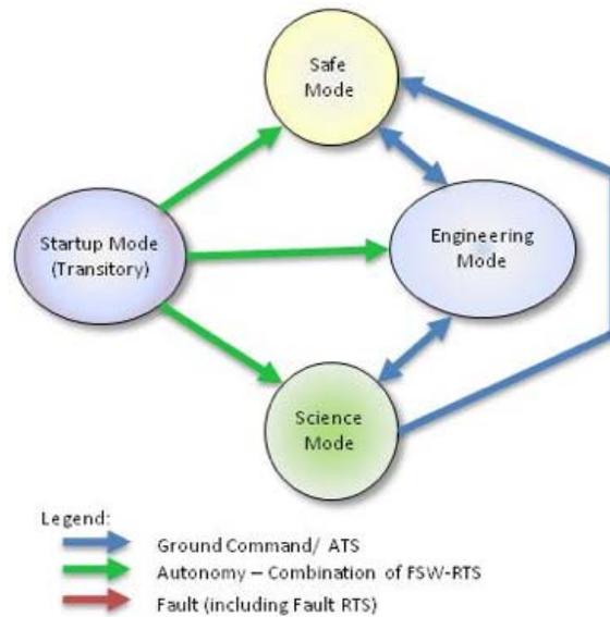
**Figure 5 - CYGNSS Observatory mode flow diagram**
