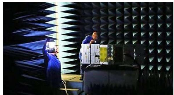
**Figure 13 - CYGNSS Observatory during L-band noise floor testing**
