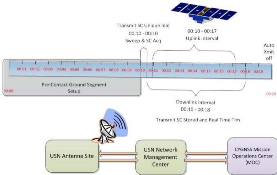
**Figure 10 - Typical CYGNSS communication pass timeline**
