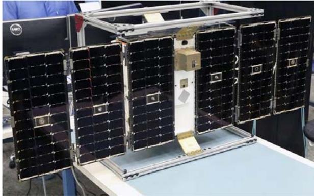
**Figure 15 -- CYGNSS Observatory Solar Array Deployment Test**
