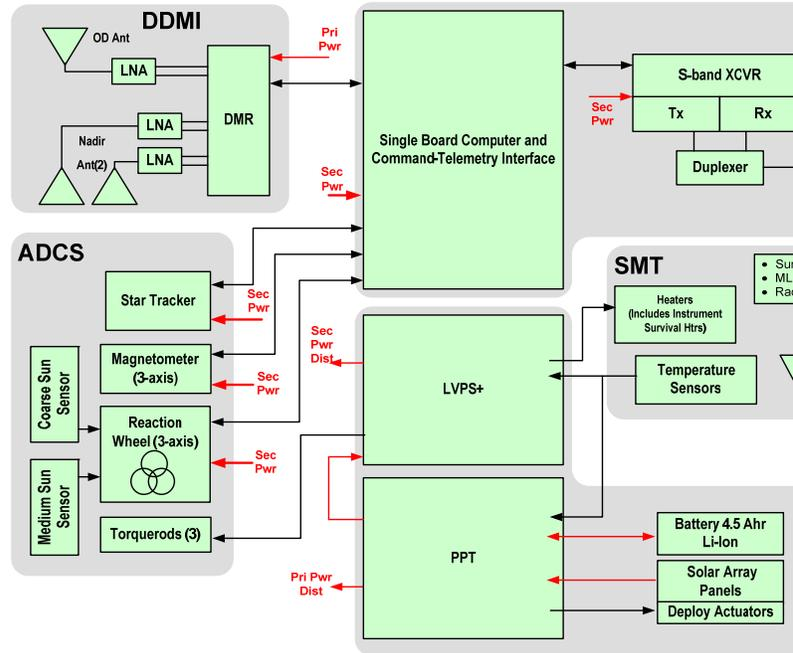
Figure 8). Due to the limited planned contact schedule as well as the limited time per contact, each uSat platform is designed and implemented to maintain the safety of the Observatory without ground intervention. The design philosophy of the CYGNSS flight segment is to maximize fault tolerance by eliminating unnecessary functionality and failure points. The CYGNSS Observatories employ a simple architecture and a simple operational schema. Redundancy is
