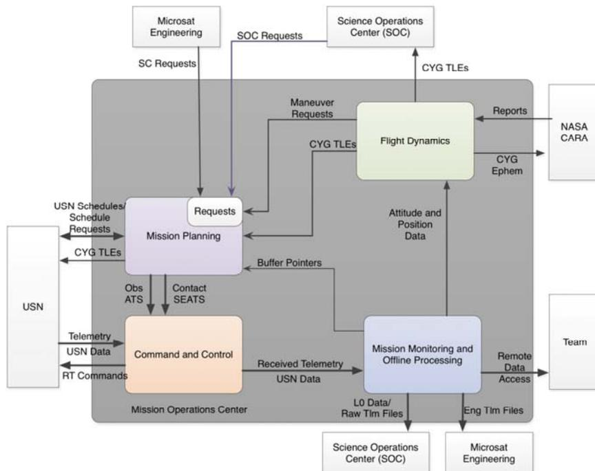
**Figure 9 - CYGNSS Mission Operations Center functional block diagram**
