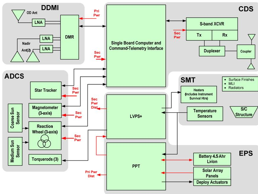
**Figure 8 - CYGNSS Observatory functional block diagram**
