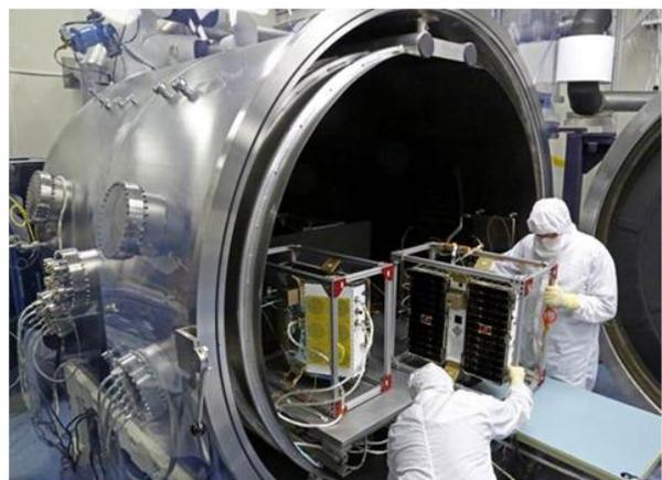
**Figure 14 - CYGNSS observatory level thermal vacuum testing**
