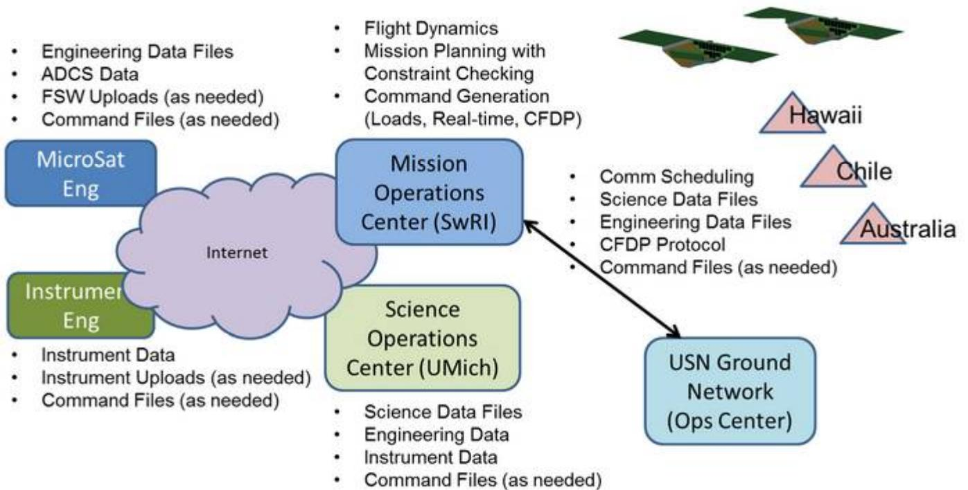
**Figure 4: CYGNSS Ground System Overview**
