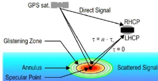
**Figure 6 Geometry for GNSS signal surface reflection showing specular point and three ellipses of constant delay**
