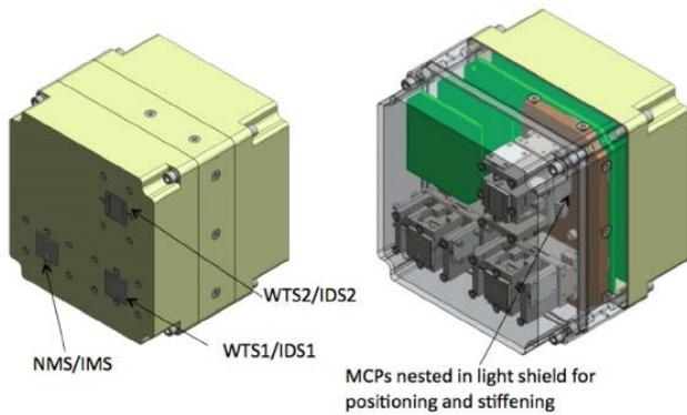
**Figure 4 Layout of the 4 WINCS spectrometers. Overall dimensions are 7.5x7.5x7.1cm<sup>3</sup>. WTS and IDS are paired in two spectrometer modules with mutually perpendicular FOV.**
