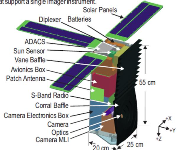
**Figure 3 The SADIE configuration closely mimics the CubeSat definition though with enlarged dimensions to accommodate the SADIE instrument. Extensive use of commercial components is exploited to reduce risk and cost**
