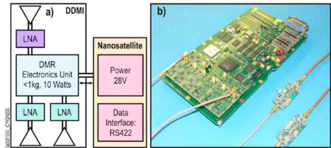
**Figure 9 (left) the GNSS instrument functional block diagram, (right) the GNSS receiver and LNAs**
