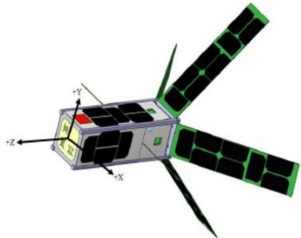
**Figure 5 The physical configuration of the Armada observatory; WINCS is on the +Z face (ram vector). Deployable solar arrays provide electrical power and passive aerodynamic stabilization**
