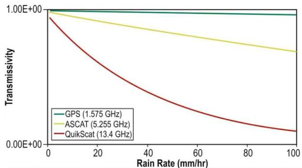
**Figure 7 Signal attenuation through precipitation**
