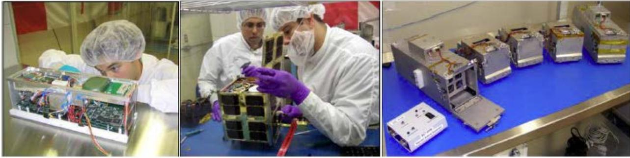
**Figure 1. (a-left) CubeSat during integration (b-center) Nanosatellite during integration, (c-right) CubeSat P-POD deployment mechanism [1]**
