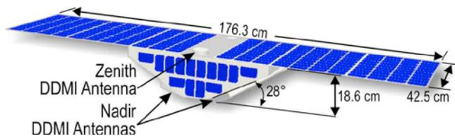
**Figure 10 The CYGNSS observatory in flight configuration**
